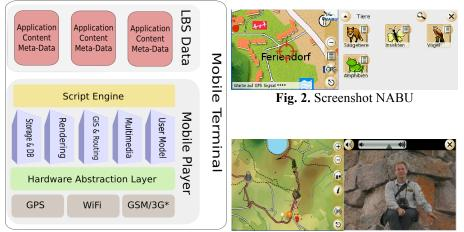
Fig. 1. Mobile Terminal's Architecture
